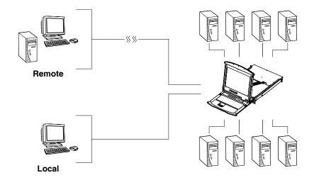
An extra console port is provided on the rear panel to manage the LCD KVM switch from an external console (monitor, keyboard, and mouse) up to 20 meters away. For added convenience, the KL9108 / KL9116 supports an external PS/2 mouse.
